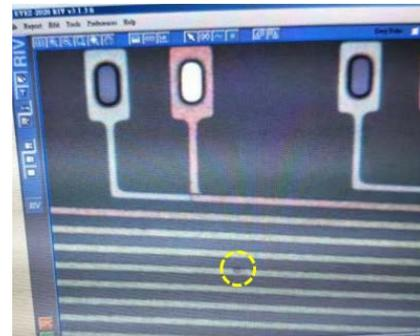
Figure 1. Overetched defect.
